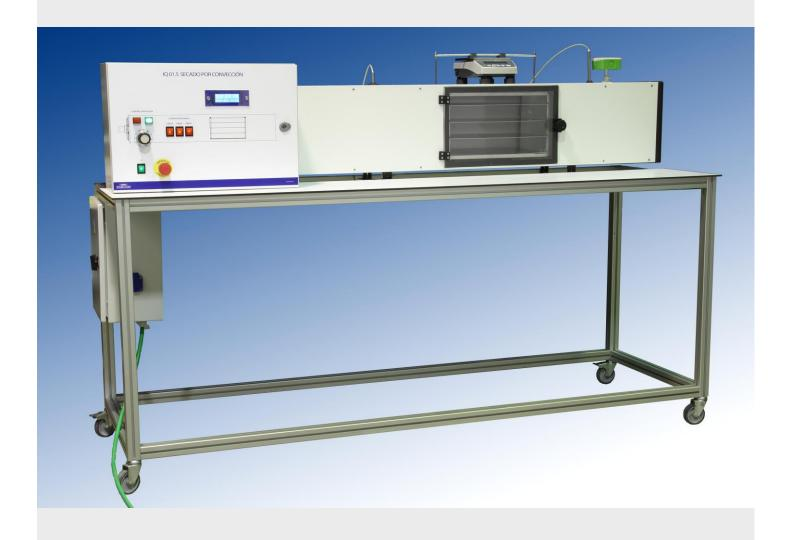
The objective of the IQ 01.5 equipment is to analyze the drying by convection of the element to be studied, modifying the environment in which it is and reflect the data of the changes produced.
