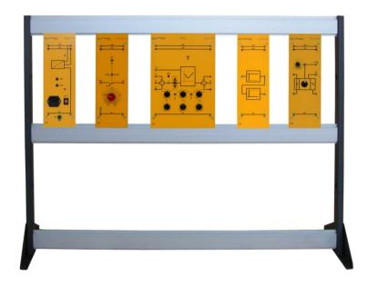
This laboratory is designed for the study of the Light Control application to allow the student a practical training, based on the performance of guided experiments. Industrial type components are educationally adapted by using a modular panel system to permit the step by step assembling from the simplest circuit to the most complex system.
