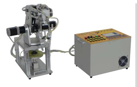
This trainer simulates the operation of an industrial robot, such as: overall rotation, arm rotation, forearm rotation, wrist rotation, gripper rotation, gripper opening/ closing.
