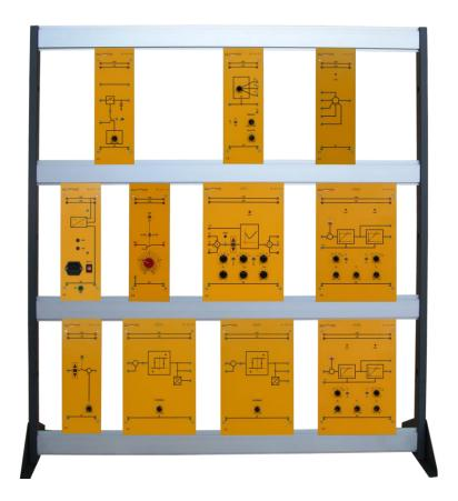
This laboratory is designed for the study of Discontinuous Automatic Control systems where the controller is composed of a an element with discontinuous intervention. A discontinuous controller is characterized by an output having two or more fixed states and its value is switched among these states according to the input value.
