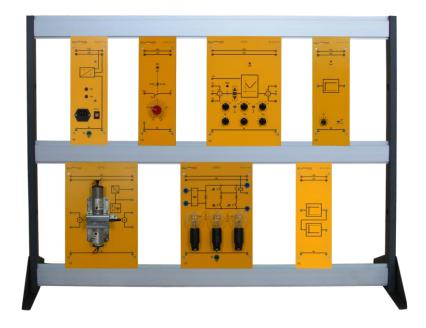
This laboratory is designed for the study of Control of a DC motor to allow the student a practical training, based on the performance of guided experiments. Industrial type components must be educationally adapted by using a modular panel system to permit the step by step assembling from the simplest circuit to the most complex system.
