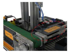
Around a PLC program, that integrates different kind of substation signals (linear transport cylinder stretch out detection, linear transport cylinder retract detection with upstream process signals and type of transported materials), it is built a transfer substation.
