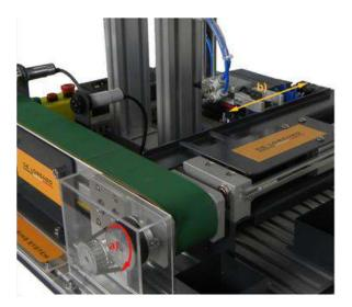
The **DL CIM-A** trainer offers an excellent possibility to study, understand, and design the most appropriate applications of a DC motor use (a). Simple, easy to control, with some proper gear, the application for belt conveyer is fast integration of this electric machine in manufacturing chain.
