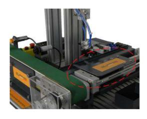
Around a PLC program, that integrates different kind of substation signals (linear transport cylinder stretch out detection, linear transport cylinder retract detection with upstream process signals and type of transported materials), it is built a transfer substation.
